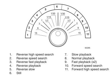
Figure 22. Shuttle Ring Speed Settings
